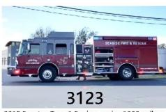
2015 Spartan Type 1 Engine carries 1000 gallons of water. First out on medical calls and motor vehicle accidents.
