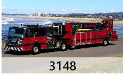
2018 Rosenbauer 100 ft Tiller Quint carries 300 gallons of water. First out on structure fires within the city and holds tech rescue equipment including Trench Rescue.
