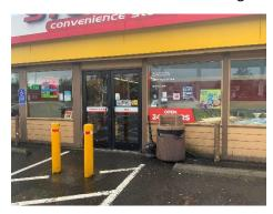
**Exit doors unlocked during business hours.** Locked exit doors make it impossible for occupants to escape safely and quickly.
