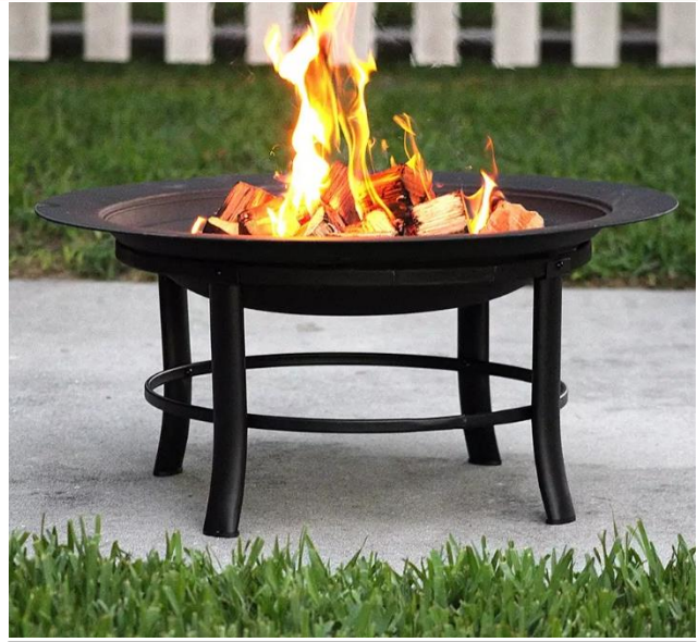
PORTABLE OUTDOOR FIREPLACE Clearances 15ft to dune grass, structures, and other combustibles, 30ft during fire season. Mineral earth, gravel, brick, or cement 15ft around fireplace, 30ft during fire season.
